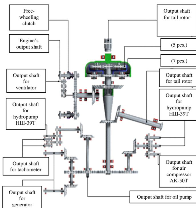
*Fig.1. Kinematic scheme of reducer BP-8(A) / BP-14*
