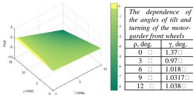
Fig.4 The dependence of the lateral displacement of the motor-grader from the angle of the front wheels tilt in the vertical plane ( $\rho$ ) and the angle of their turning in the horizontal plane ( $\gamma$ ). The working operations are performed on the site with transverse gradient of  $\varphi=8^\circ$ .
