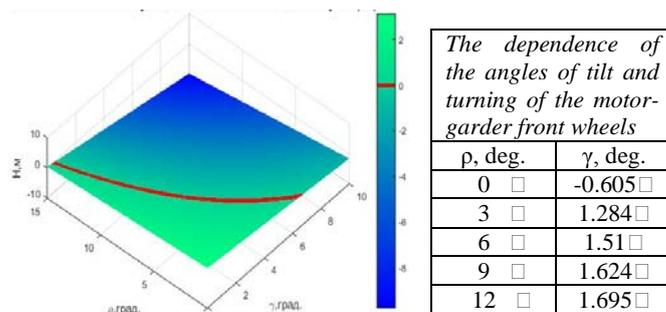
Fig.3 The dependence of the lateral displacement of the motor-grader from the angle of the front wheels tilt in the vertical plane ( $\rho$ ) and the angle of their turning in the horizontal plane ( $\gamma$ ).
