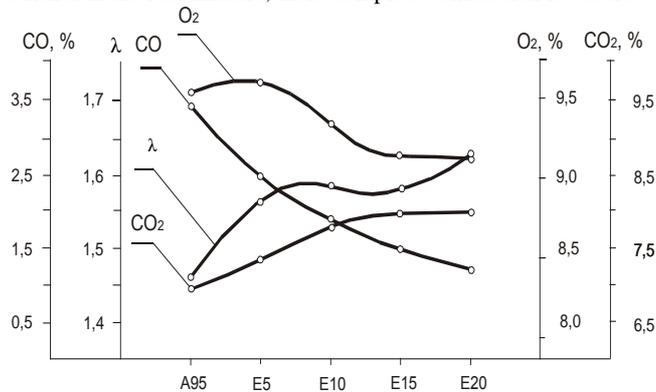
**Picture 4.** Dependence of carbon monoxide content (CO), carbon dioxide ( $\text{CO}_2$ ), oxygen ( $\text{O}_2$ ) and the excess air factor  $\lambda$  from the ethanol content ( $n = 1000 \text{ min}^{-1}$ ).
