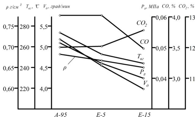
**Picture 3.** The main characteristics of engine from fuel mixture
