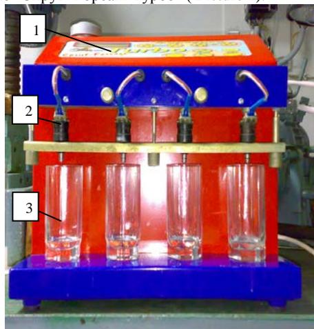
**Picture 1.** Stand «Спрут-Форсаж-Турбо»: 1 – control panel; 2 – injector; 3 – glass for the fuel collection.
