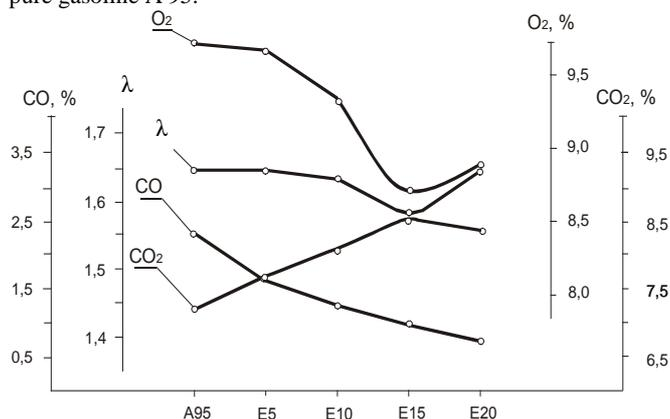
**Picture 5.** Dependence of carbon monoxide content (CO), carbon dioxide ( $\text{CO}_2$ ), oxygen ( $\text{O}_2$ ) and the excess air factor  $\lambda$  from the ethanol content ( $n = 2000 \text{ min}^{-1}$ ).
