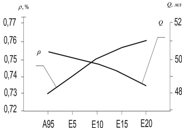
**Picture 2.** Dependence density fuel-mixed  $\rho$  and the amount of fuel  $Q$  injected from its composition.
