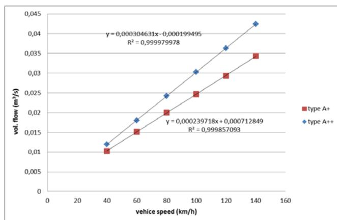
**Fig. 11** Comparison of volumetric flow type A+ and A++
