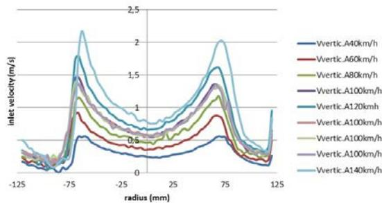
Fig. 5 Comparison of velocity profiles at different rotational speeds.
