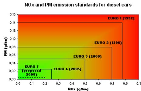
Fig. 2 Emission standards for NO<sub>x</sub> and PM of diesel cars.
