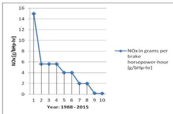
**Fig.3** NO<sub>x</sub> reduction of emissions in the period 1988-2015 year.
