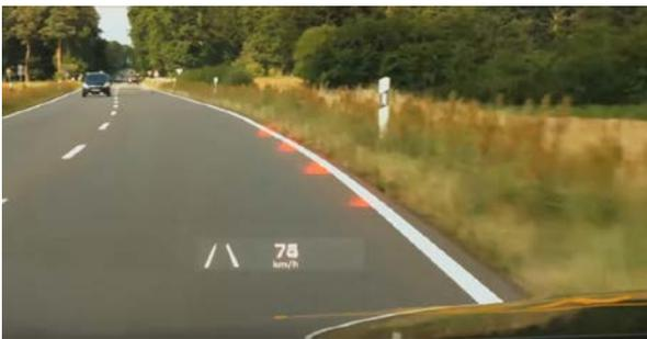
**Fig. 2** Driver Assistance System for lane keeping
