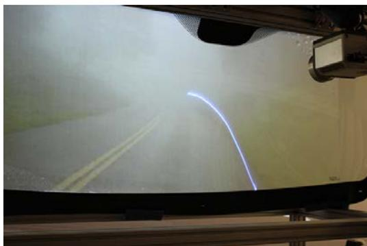
**Fig. 3** Driver Assistance System for lane keeping
