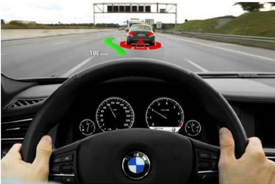
**Fig. 1** Driver Assistance System for lane departure
