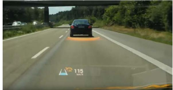
**Fig. 4** Driver Assistance System for obstacle detection on the road
