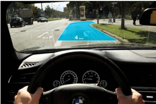
**Fig. 7** Driver Assistance System for navigation
