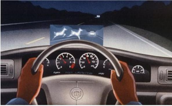
**Fig. 6** Driver Assistance System for night vision
