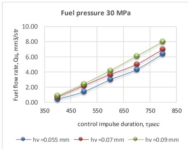
Fig. 6 Alteration of the fuel flow rate defined by the stroke of the control ball valve  $h_v = 0.055 \div 0.09$  mm
