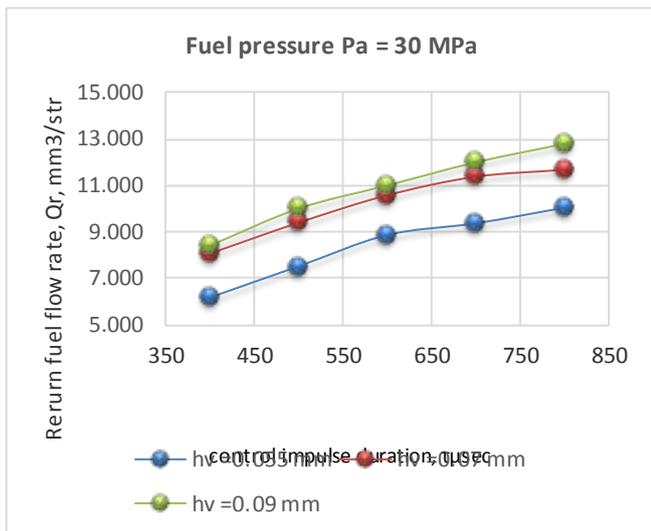
Fig. 7 Alteration of the returned fuel flow rate defined by the stroke of the control ball valve  $h_v = 0.055 \div 0.09$  mm
