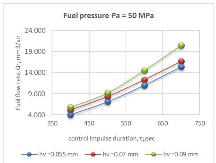
Fig. 11 Alteration of the returned fuel flow rate defined by the stroke of the control ball valve  $h_v = 0.055 \div 0.09$  mm
