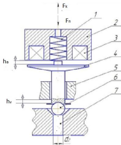
Fig. 2 General appearance of the solenoid:
