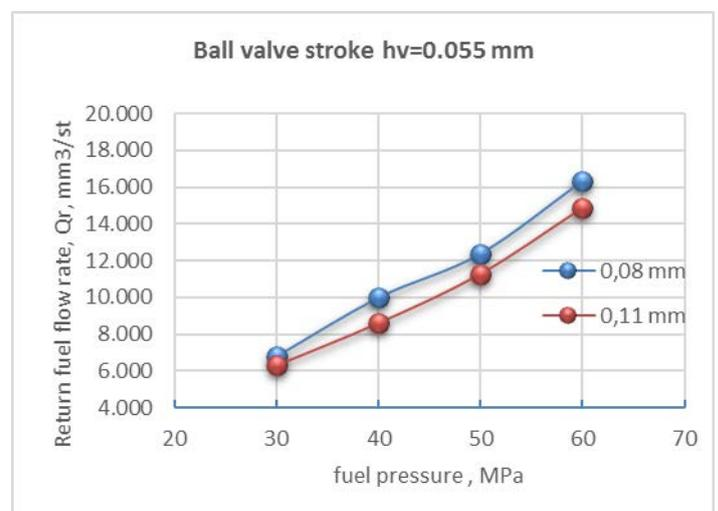
Fig. 5 Alteration of the return fuel flow rate defined by the magnitude of the electromagnetic gap  $h_{coil} = 0.08 \div 0.11$  mm in the control valve and the fuel pressure  $P_a = 30 \div 60$  MPa
