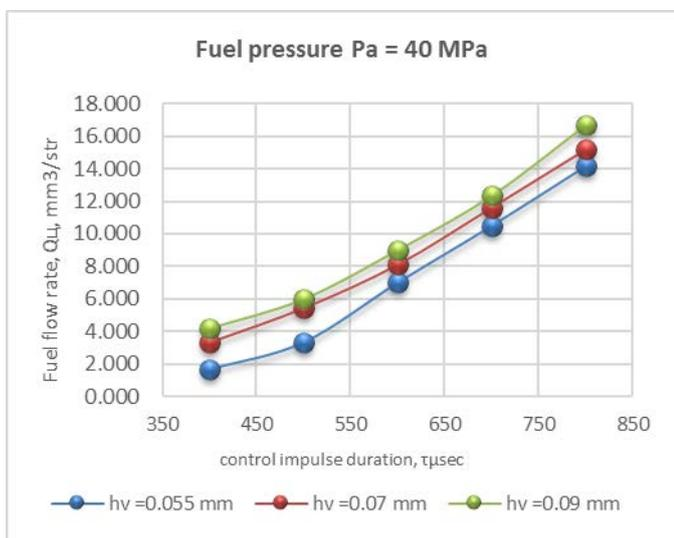
Fig. 8 Alteration of the fuel flow rate defined by the stroke of the control ball valve  $h_v = 0.055 \div 0.09$  mm
