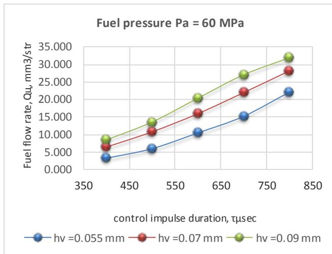
Fig. 12 Alteration of the fuel flow rate defined by the stroke of the control ball valve  $h_v = 0.055 \div 0.09$  mm
