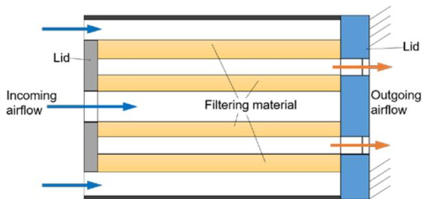
Fig. 4 Computational schema for airflow calculation
