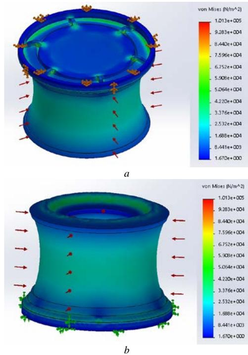
Fig. 10 Distribution of stresses in a double-layer construction in a round-shaped air filter: a) top view; b) bottom view
