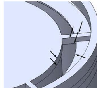
Fig. 6 Sharp edges of air filter lid
