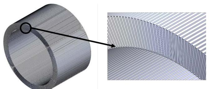
Fig. 2 3D model of pleated filtering material of round-shape outer ring
