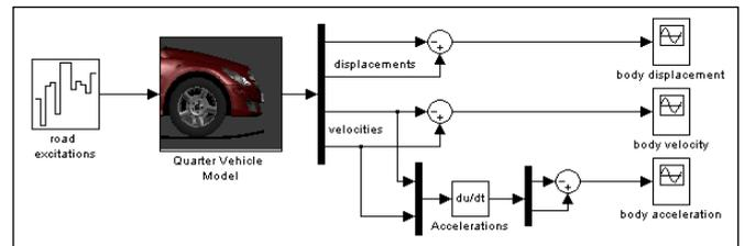
Fig 2. Simulation scheme of Quarter Vehicle Model
