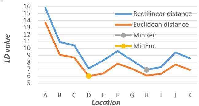
Fig. 3 Comparison of the results for Euclidean and rectilinear distance calculation in load distance method.
