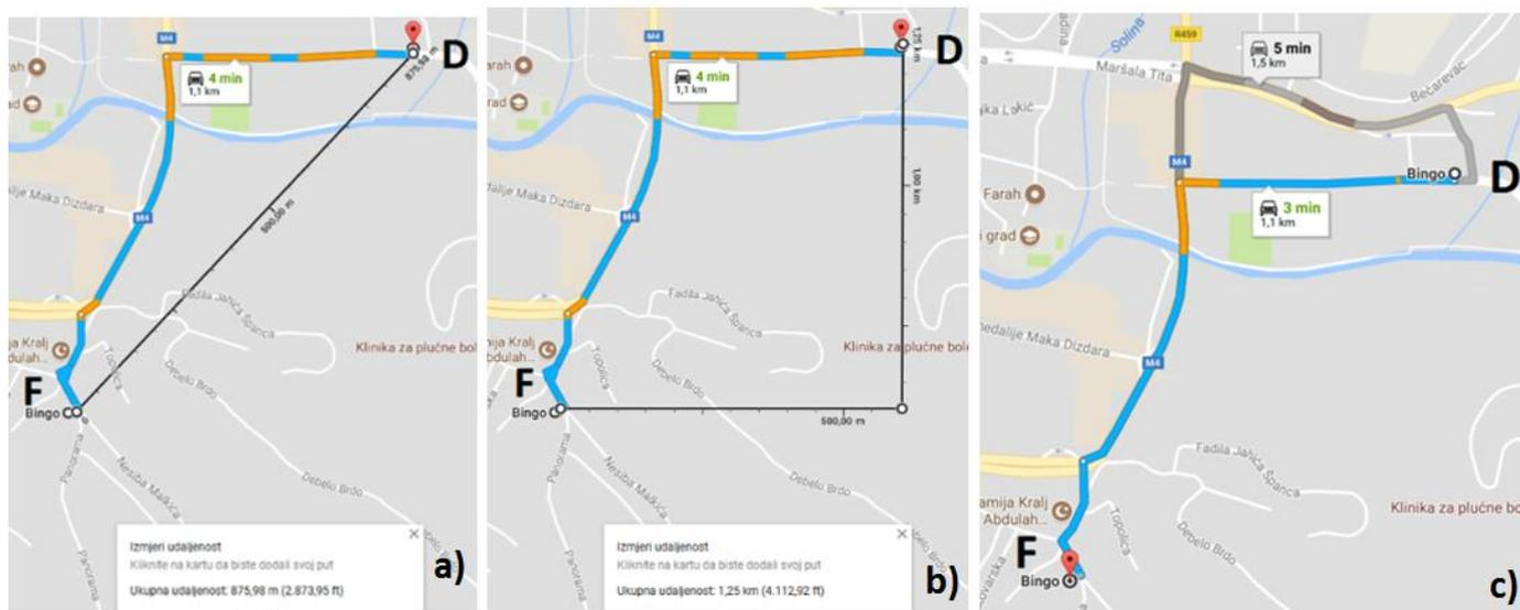
Fig. 4 Different ways to determine  $D_{ij}$  distance between two potential locations: a) Euclidean distance:  $D_{ij}=0,875$  [km], b) rectilinear distance:  $D_{ij}=1,25$  [km], c) real distance determined by transport routes:  $D_{ij}=1,1$  [km].
