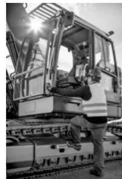
Fig. 1. Support points on the inside of the excavator's cabin [1]
