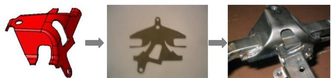
Fig. 3 Process of prototyping the complex element.
