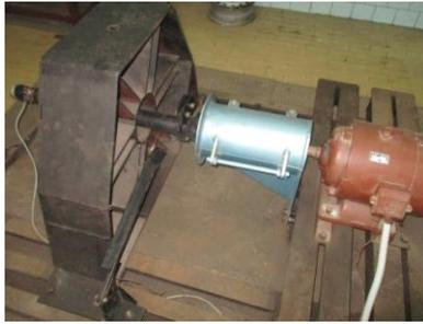
**Fig. 6** Position of load weights and automatic shutting down system in the event of increased amplitudes of oscillation
