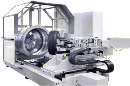
Fig. 2 ZWARP testing bench by MAKRA company
