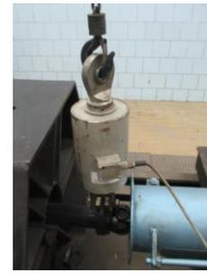
**Fig. 8** Calibration of strain gauges in the shaft using HBM force transducer
