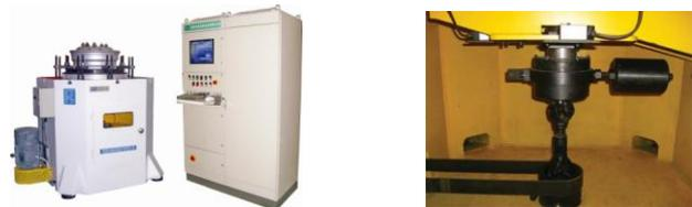
Fig. 1 CFT-5 testing bench with a detailed overview of the rotating weight
