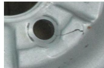
**Fig. 9** Typical fracture on a wheel disk
