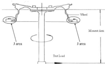
Fig. 4 Centrifugal force testing
