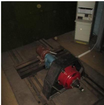
**Fig. 7** Testing bench for wheel testing complete with measurement-control unit
