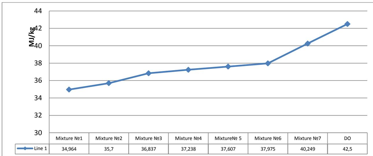
It can be seen that the high content of alcohol significantly influences the reduction of the heat of the fuel combustion, for example, a mixture of 80% DO and 20% RicO has a combustion heat of 40.986 MJ / kg, and a similar mixture with an alcohol of 80x10x10 already has 40.24 MJ / kg. Due to the addition of bioethanol, the
