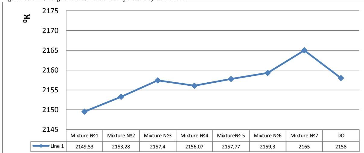
Increasing the proportion of bioethanol also affects the combustion temperature. According to calculations, it was revealed: the lower the amount of diesel fuel is and the higher the amount of alcohol is, the lower the combustion temperature of the mixture is. But with the addition of not more than 25% of the biocomponents, the combustion temperature rises according to the made calculations.
