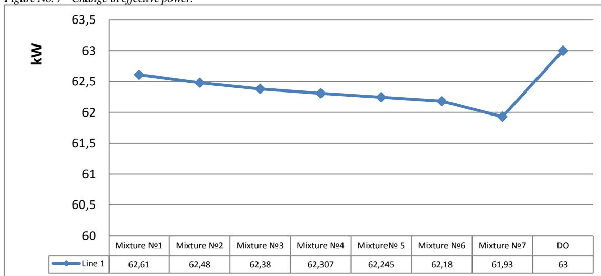
But the presence of alcohol favorably influences the performance of ICE, so based on the obtained data on the example of mixtures with a 60% content of DO, it is evident that when the alcohol content is changed by 5%, the effective power increases on the 62-70 W.
