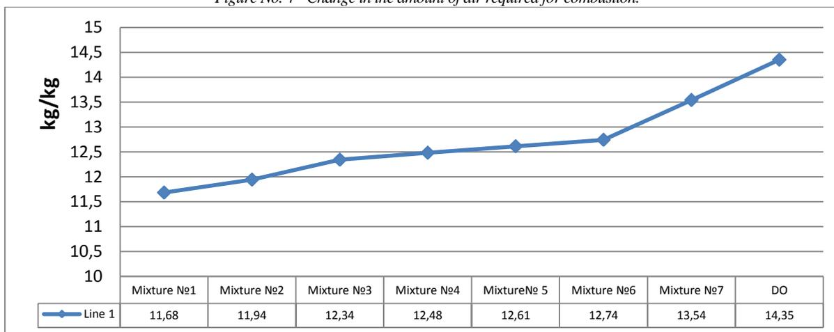
An important feature of the addition of bioethanol in diesel composite fuel mix is the reduction in the required amount of air for firing 1 kg of fuel. From this it can be concluded that for the transfer of the diesel internal combustion engine (ICE) with the system without adjusting the amount of air supplied, it is necessary to modernize the air supply system of the internal - combustion engine.
