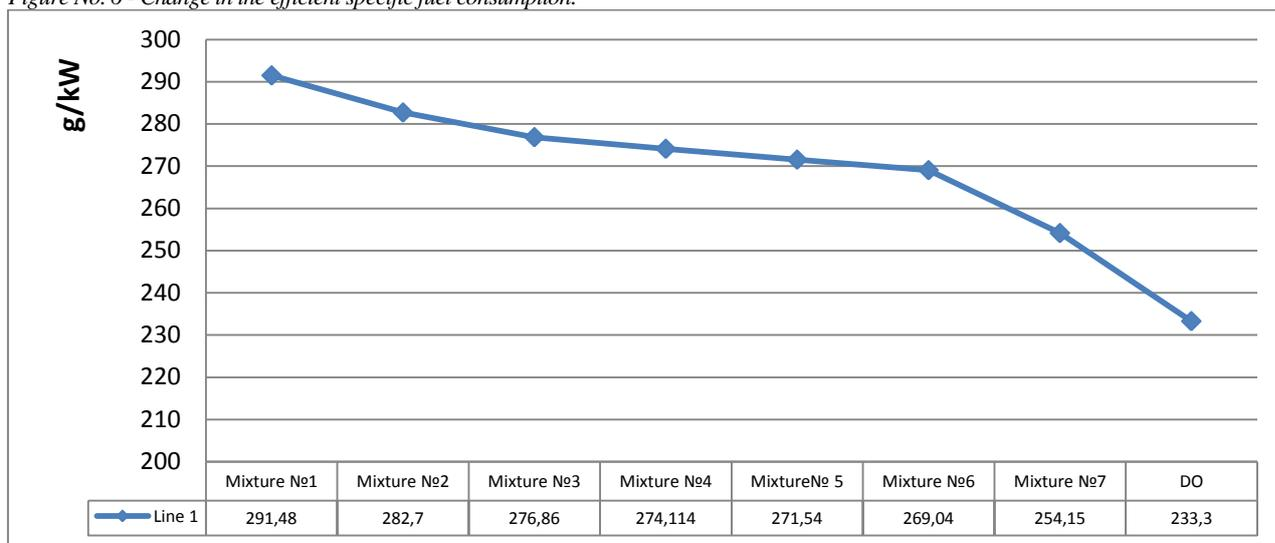
According to the schedule, a significant increase in the specific fuel consumption is affected by an increase amount of bioethanol.
