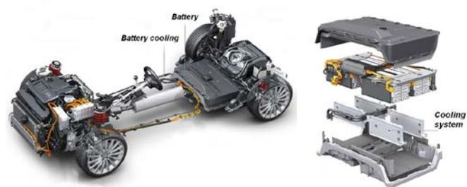
**Fig. 3** High-voltage car battery Audi A3 e-tron PHEV-20.
