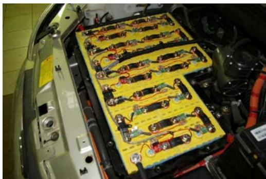
Fig. 5 High-voltage car battery LADA Ellada.
