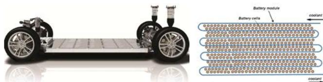
Fig. 4 High-voltage car battery Tesla Model S.
