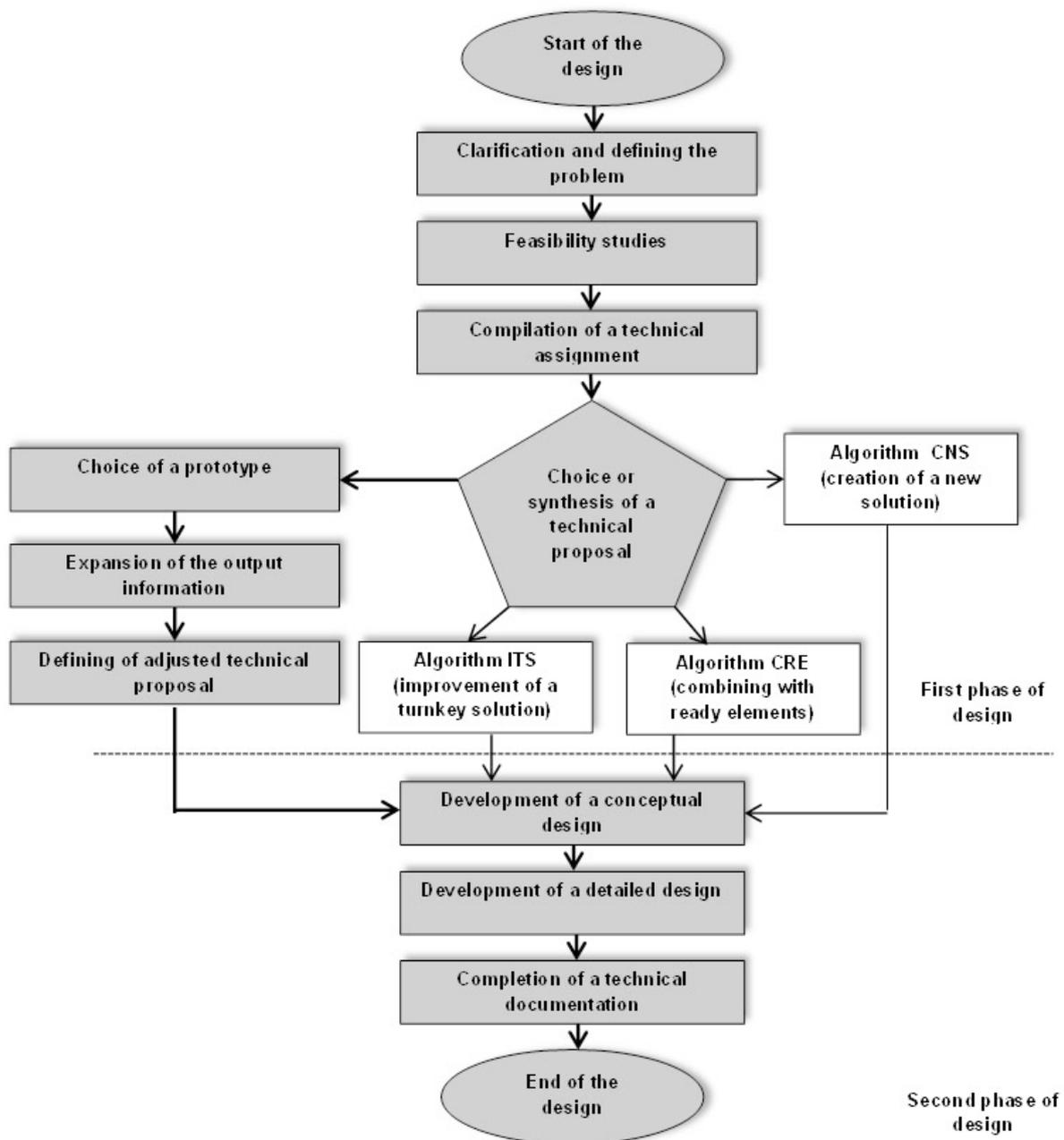
Fig. 2 A model (algorithm) for solving the engineering problem of adapting of an existing (turnkey) solution to work in new conditions
