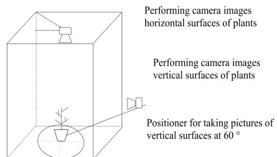
Fig. 1 The scheme of the test site
