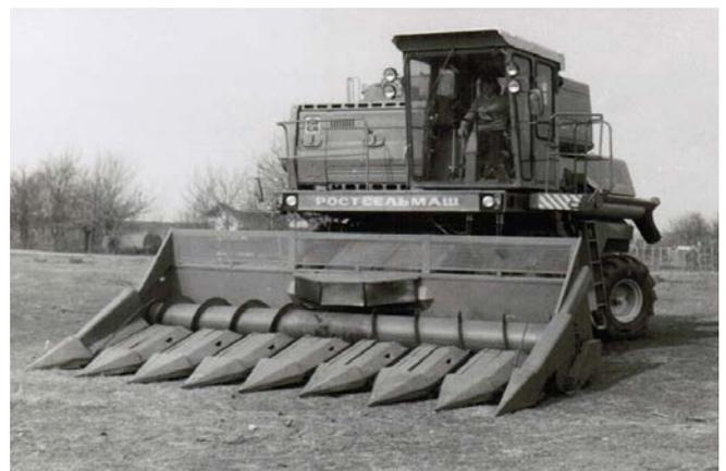
Fig. 1 Row header for harvesting soybeans HS
