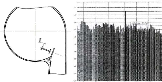
fig. 15. Petalled activator of interaction of flows in the volute and the amplitude-frequency characteristics
