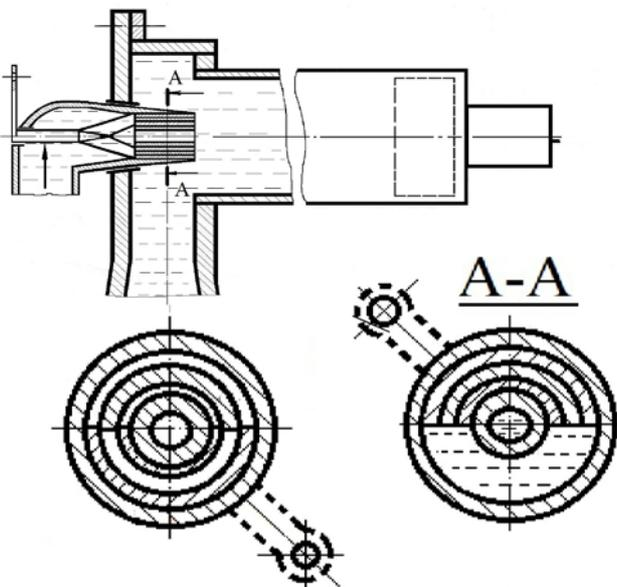
fig. 9. Axial input of the transit flow through the multislit nozzle
