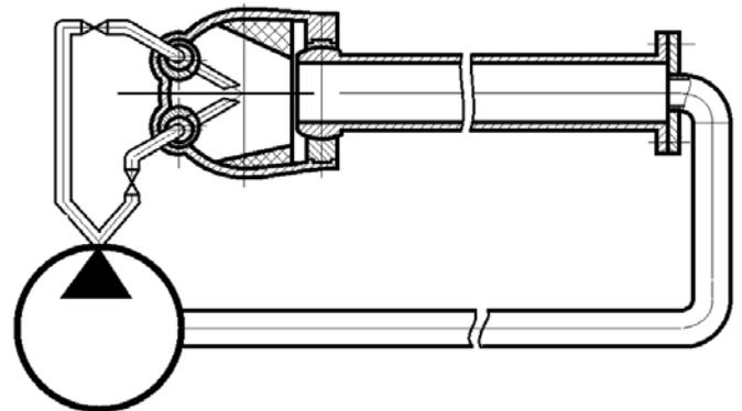
fig. 12. Irrotational hydrodynamic cavitator
