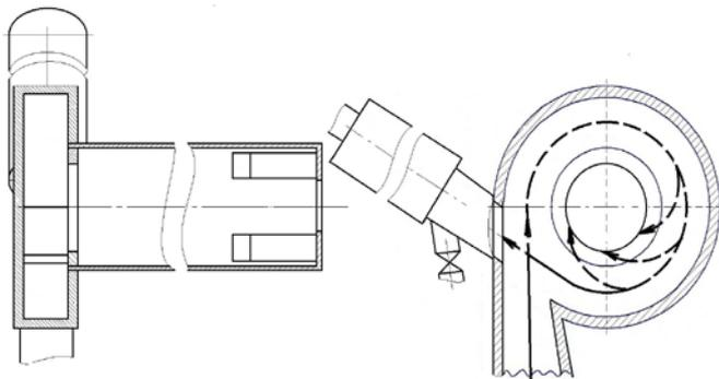
fig. 14. Vortex cavitator with intersecting streams
