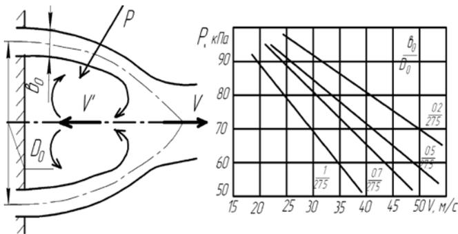
fig. 13. Creating an acoustic signal by periodically destroying dome
