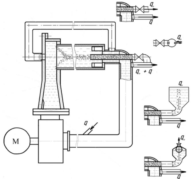
fig. 11. Collecting the evolved gas at the outlet of the body of the cavitator
