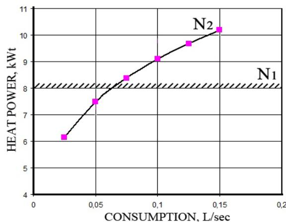
fig. 3. Thermal efficiency of the cavitator
