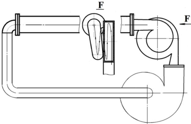
fig. 8. The construction of the vortex cavitator with straightening of the flow at the output of the snail
