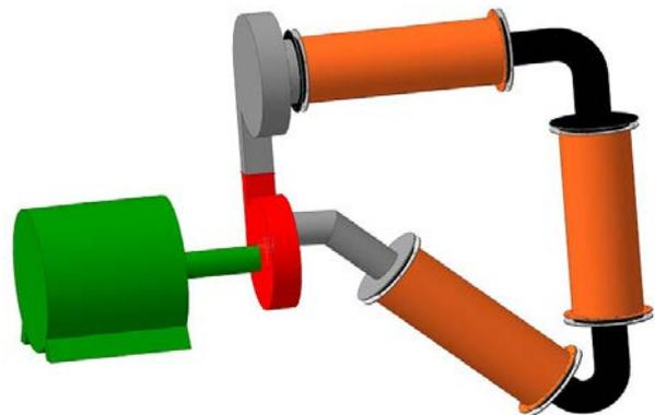
*fig. 7. Multihull option of a hydrodynamic cavitator*
