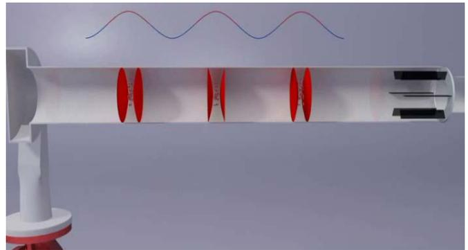
*fig. 6. Body of the cavitator with a standing wave*
