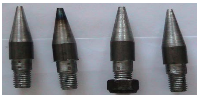
Figure 2. A spike- tooth that used for threshing unit.
