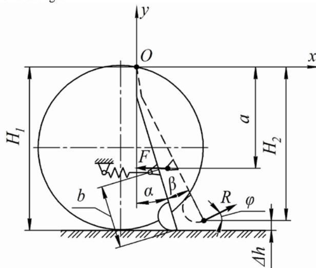
Fig. 2. Equivalent scheme of the combined two-disc anchor opener
