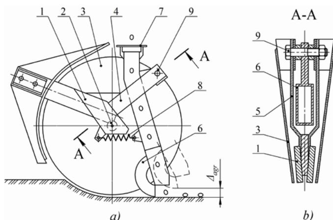
Fig. 1. Structural scheme of the combined two-disc anchor opener: a) – side view when removing the left disk; b) – section along A-A: 1 – case; 2 – axle; 3 – disk; 4 – holder; 5 – plate; 6 – opener tip; 7 – socket; 8 – spring; 9 – hinged suspension
