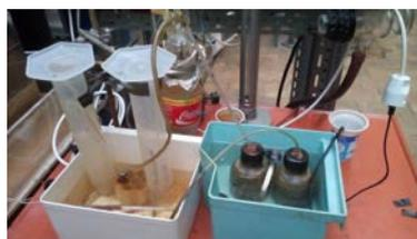
Fig. 1 Outlook of the small scale bioreactor
