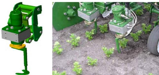
Fig. 9. Cultivator with automatic rotating knives.
