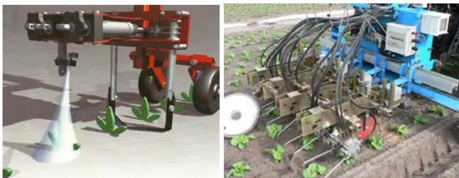
Fig. 8. Cultivator with automatic diverting knives.
