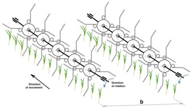
Fig. 7. Scheme of working organs of a cultivator with rotating bodies with spring metal fingers.
