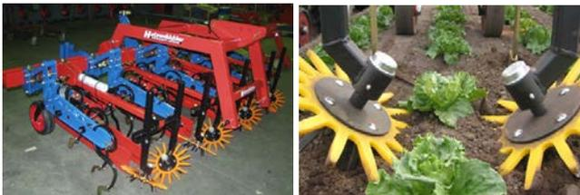
Fig. 5. Cultivator for hoeing with rotating teeth bodies with passive action.
