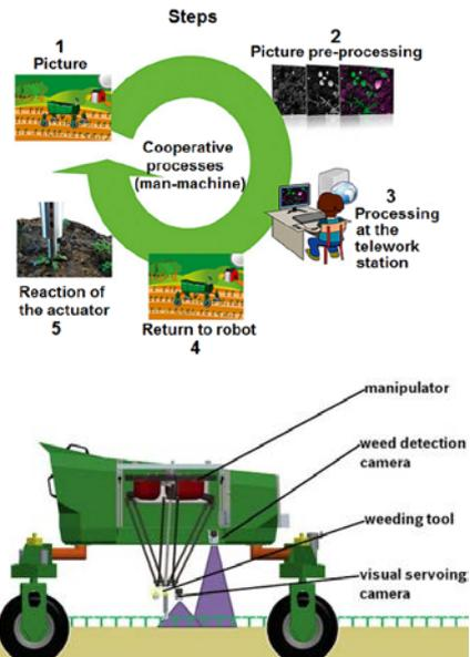
Fig. 10. Web-based robot assisted secondary vegetation control.
