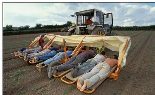
Fig. 2. Tractor platform for manual weeding.
