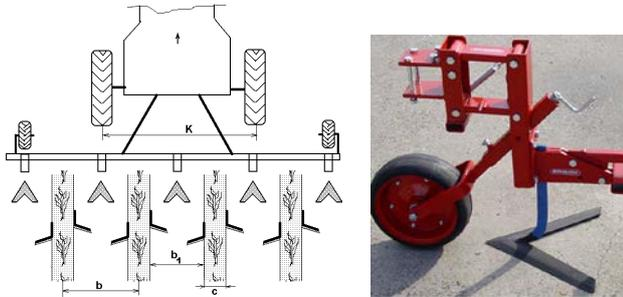
Fig. 3. Scheme of the cultivator for row cultivation and working section: *c* - protection zone; *b* - spacing between the rows; *b<sub>1</sub>* - processed area; *k* - distance between the wheels of the tractor.
