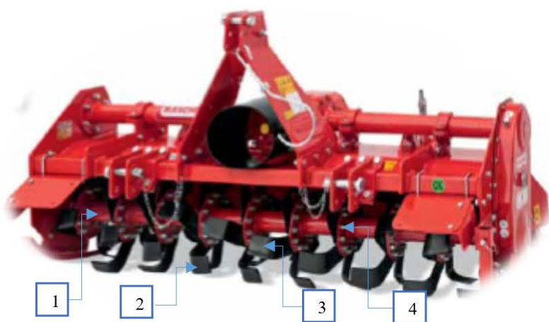
Fig. 1. MASCHIO H205 rotavator with 10 flanges and 60 blades; 1 - rotor, 2 - right blade, 3 - left blade, 4 - flange (on the left); The tiller blade 1 and 2 in study, from two different manufacturers made from two different steels brands, 'C' shaped & 'H' type [3].
