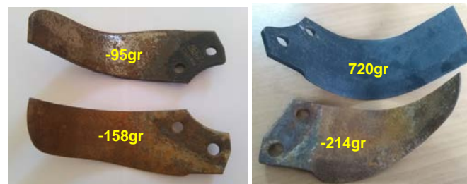
Fig. 3. Wear tiller blades 1 and 2, after tillage of 45 hectares (on the left) and blade 2 (on the right) as new product that weight 720gr, under it the same blade with full wear at the end of its lifecycle.
