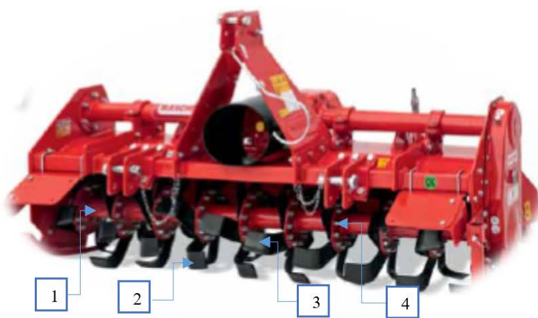
Fig. 1. MASCHIO H205 rotavator with 10 flanges and 60 blades; 1 - rotor, 2 – right blade, 3 – left blade, 4 – flange (on the left); The tiller blade 1 and 2 in study, from two different manufacturers made from two different steels brands, 'C' shaped & 'H' type [3].
