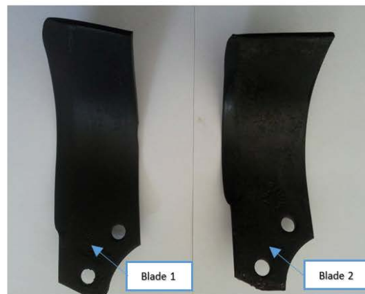
Fig. 1. MASCHIO H205 rotavator with 10 flanges and 60 blades; 1 - rotor, 2 – right blade, 3 – left blade, 4 – flange (on the left); The tiller blade 1 and 2 in study, from two different manufacturers made from two different steels brands, 'C' shaped & 'H' type [3].
