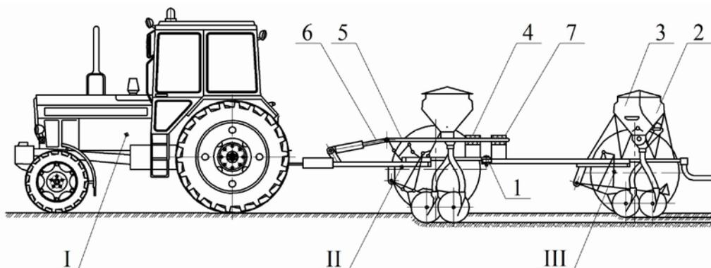
**Fig. 1.** Unit for underground soil mineral fertilizer and simultaneous sowing of grain crops (side view):
