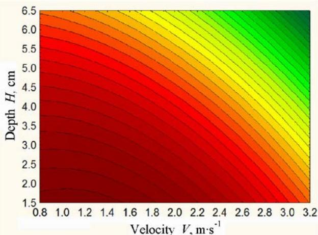
**Fig. 8.** Effect of the forward speed of the fertilizer-seeding unit and the depth of sowing of seeds on the two-dimensional cross-section of the coefficient of variation of the depth of sowing of barley seeds
