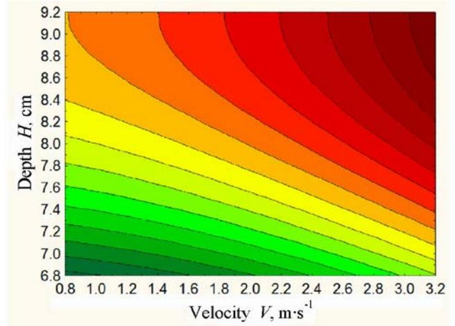
**Fig. 5.** Two-dimensional section of the dependence of the uniformity of the distribution of fertilizers (soybean seeds) along the row on the speed of movement of the fertilizer-seeding unit and the depth of fertilization in the soil
