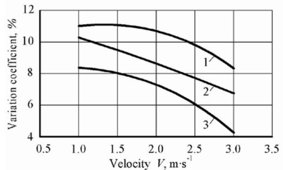
**Fig. 6.** Effect of the forward speed of the fertilizer-seeding unit on the variation coefficient of the depth of sowing of barley seeds at a different depths of seed sowing: 1 – H = 2 cm; 2 – H = 4 cm; 3 – H = 6 cm
