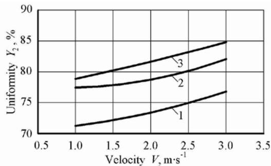
**Fig. 3.** The effect of the speed of the fertilizer-seeding unit on the uniformity of the distribution of fertilizers (soybean seeds) along the line at a different depths of laying fertilizers in the soil: 1 – H = 7 cm; 2 – H = 8 cm; 3 – H = 9 cm
