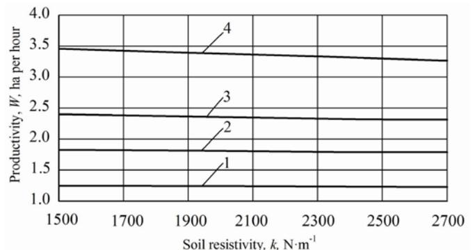
Fig. 3. – Dependence of the efficiency  $W$  of the top removal machine frontally mounted on the wheeled tractor, traction class 3, on the specific resistance  $k$  at various working widths  $B$ :
