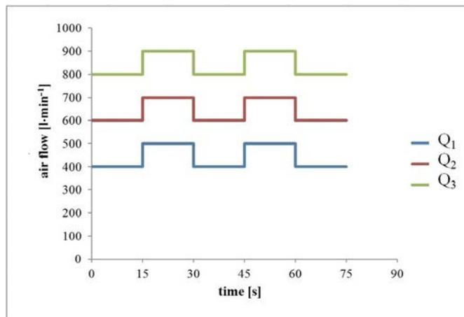
Fig. 2 Variable flow rate of air sucked in by the milking machine
