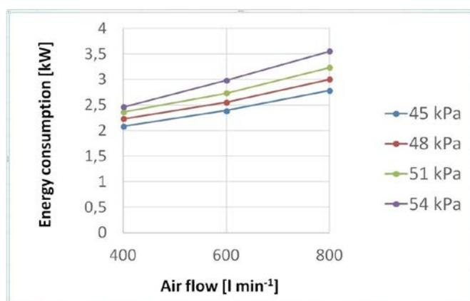
Fig. 4 Energy consumption of vacuum pump electric motor
