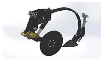
Fig. 9. Fixed suspension on spring stand
