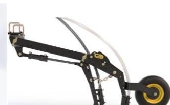
Fig. 10. Single hinge suspension
