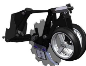
Fig. 1. Sowing section with cross slot seed boot
