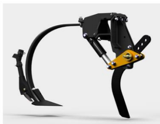
Fig. 3. Seeding section with baker boot and a cutting blade before it
