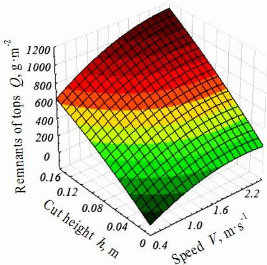
Fig. 4. – The response surface of the dependence of tops remnants on root crop head surface on the speed of movement of tops harvesting machine and the cut height at a rotor speed of 1000 rpm
