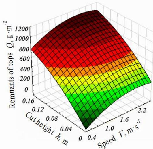
Fig. 3. – The response surface of the dependence of tops remnants on root crop head surface on the speed of movement of tops harvesting machine and the cut height at a rotor speed of 500 rpm
