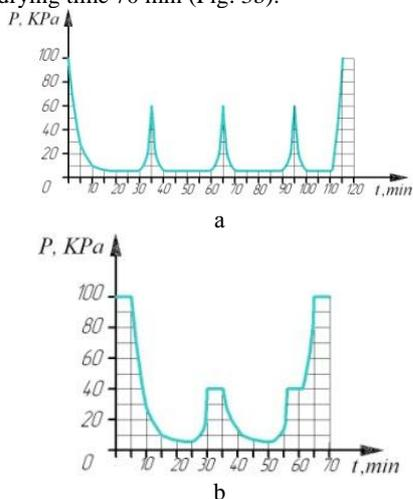
**Fig. 3.** — The pressure change in the surrounding space by direct evacuation seeds of crops: a — partial blowing mode of seeds and increased pressure to 60 kPa; b — blowdown mode for 10 min at 40 KPa
