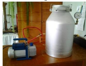
**Fig. 1.** – The construction scheme (a) and general view (b) of the experimental plant for the study of vacuum drying of seeds of crops: 1 – vacuum chamber; 2 – rotary vane vacuum pump subzero to the vacuum; 3 – faucet of a vacuum pump; 4 – faucet for throwing down of vacuum; 5 – vacuum-gauge; 6 – cover with gasket; 7 – locking mechanism; 8 – frequency converter; 9 – power supply.
