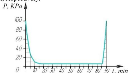
**Fig. 2.** – Change in pressure in the environment during the direct evacuation of grain seeds
