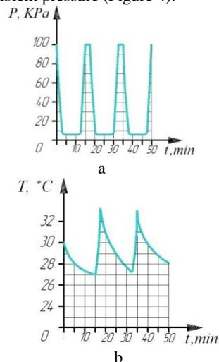
**Fig. 4.** – The change in the ambient pressure (a) and the heating temperature of the seeds (b) during the periodic heating and evacuation of seeds of cereals
