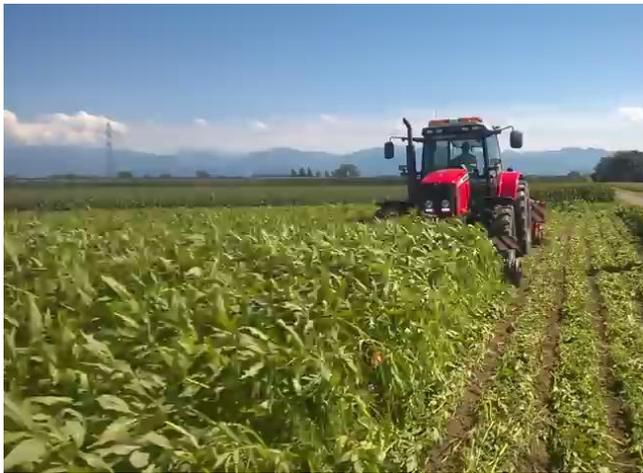
Fig. 3. Strip tilling of the soil for green crops - front view
