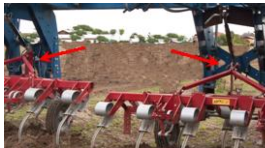
Fig. 1. Hitch linkages of wide span tractor ASALift WS9600
