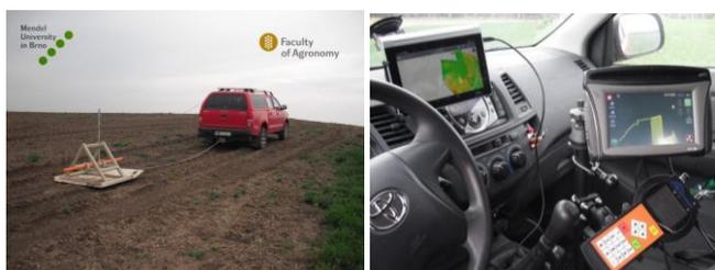
Fig. 2 Measurement of soil EC by GF Instruments CMD devices.
