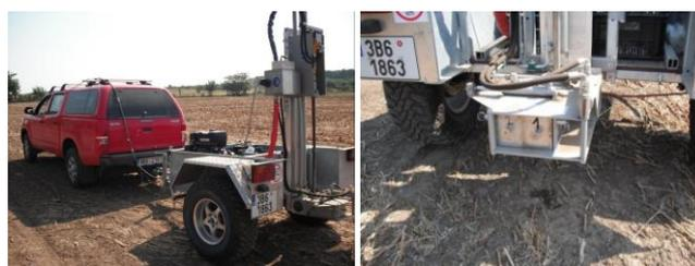
Fig. 1 Soil sampling by automatic sampler Nietfeld Duprob 60.
