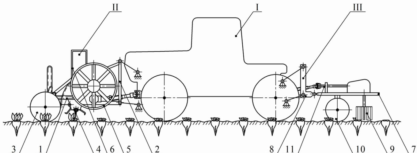
**Fig. 1.** – Combined machine-tractor aggregate for the harvest of the sugar beet heads:
