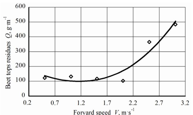
Fig. 2. – Effect of the forward speed of the machine at a rotor speed of 1000 rpm and a height of cut of 0.02 m on a amount of the residues of the sugar beet root tops on the head of roots
