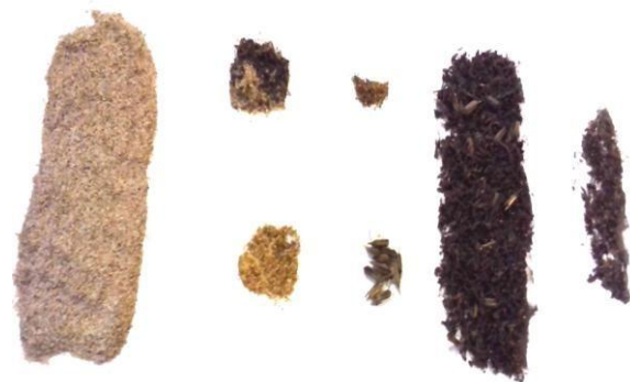
Fig. 18 Components from threshing stems in the bag of the inertial thresher
