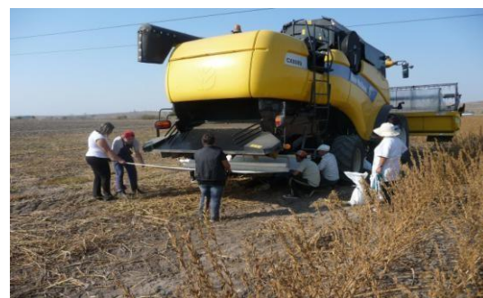
Fig. 10 Two self unscrew canvases for collecting samples from the cleaner and from the straw walker
