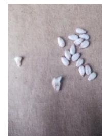
Fig. 8 Seeds damaged by the shock impulse
