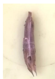
Fig. 7 A capsule damaged by a shock impulse
