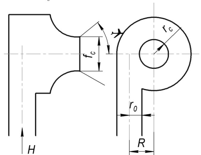
Fig. 3. – The scheme of the centrifugal nozzle. [1]
