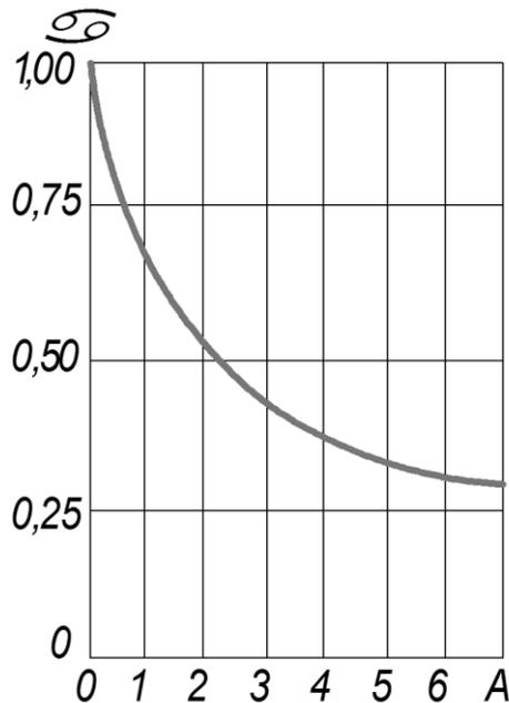
Fig. 4. – Dependency curve  $\alpha$  from  $A$  for centrifugal nozzle
