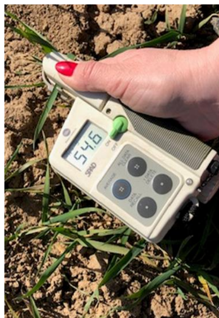
Fig. 1. Determination of chlorophyll content in leaves with SPAD 502.
