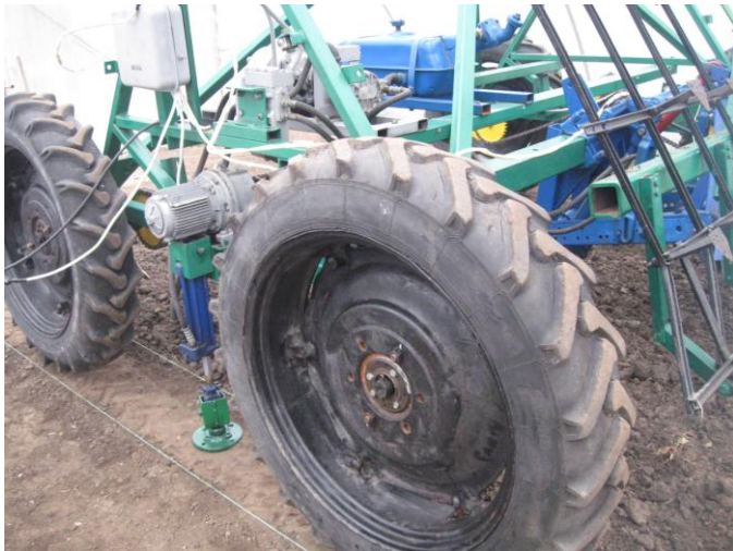
Fig. 2. Specialised Broad Track Agricultural Unit with hydraulic support for the implementation of on-board turning
