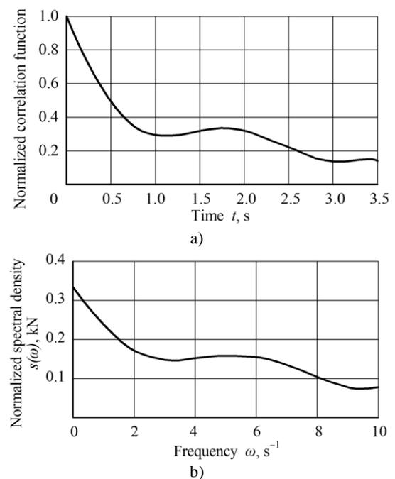
**Fig. 3.** Graphs of the normalized correlation function (a) and spectral density (b) of oscillations of the traction resistance of the harrowing tool
