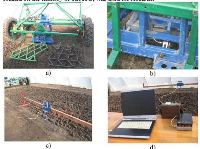
**Fig. 1.** The studied agricultural bridge harrowing unit (a); dynamometer (b); automated profilograph (c); analog-to-digital converter (ADC) and PC (d)
