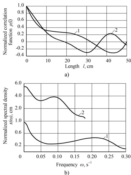
**Fig. 2.** Graphs of the normalized correlation function (a) and the spectral density (b) of the inequalities of the longitudinal profile of the traces of the constant technological track (1) and the harrowed agricultural background (2)
