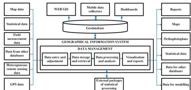
Fig. 1. Structural-functional model of GIS crop monitoring remote sensing system
