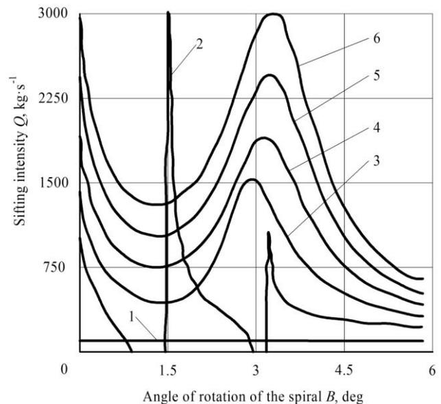
**Figure 3.** Dependence of sieving intensity  $Q$  (kg·s<sup>-1</sup>) from the angle of rotation of the spiral  $B$  (deg) at the angular velocity of the spiral: 1 – 0 rad·s<sup>-1</sup>; 2 – 10 rad·s<sup>-1</sup>; 3 – 20 rad·s<sup>-1</sup>; 4 – 30 rad·s<sup>-1</sup>; 5 – 40 rad·s<sup>-1</sup>; 6 – 50 rad·s<sup>-1</sup>
