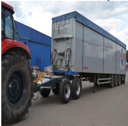
Fig. 5. NPS 3250 grain truck semi-trailer with PSP-20 saddle trailer for work with a tractor in the field
