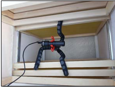
Fig. 2. Installation of the microphone inside the beehive
