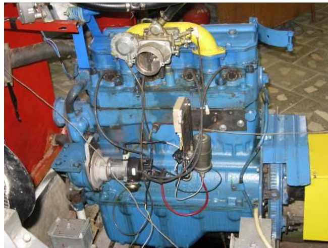
Fig. 1. Converted D-243 diesel engine into a gas engine on the test stand
