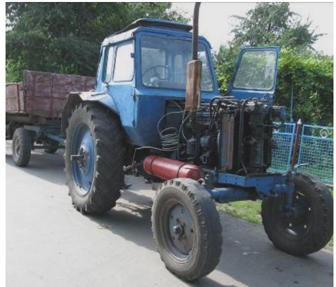
Fig. 3. Wheel tractor MTZ-80 with a diesel-to-gas converted engine
