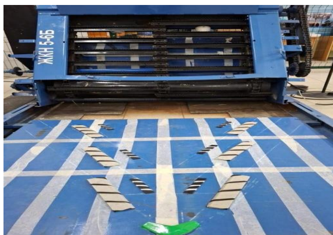
Figure 3 – Laboratory samples of threshing activators Note – compiled by the authors based on the source [1,2]
