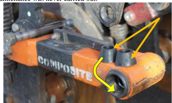
Fig. 6 - Experimental parts 1 made of carbon plastic after inspection at 400 hours of operation.
