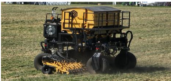
Fig. 1- The world's first autonomous agricultural robot DOT (before CNH's purchase).
