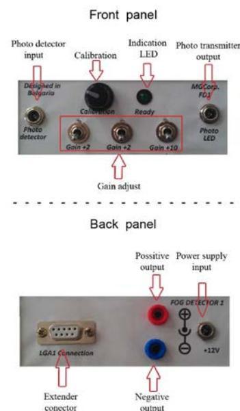
Fig. 5 – Mechanical description and connection diagram
