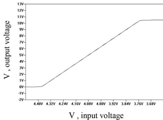
Fig. 4 – Electrical simulation with maximum gain
