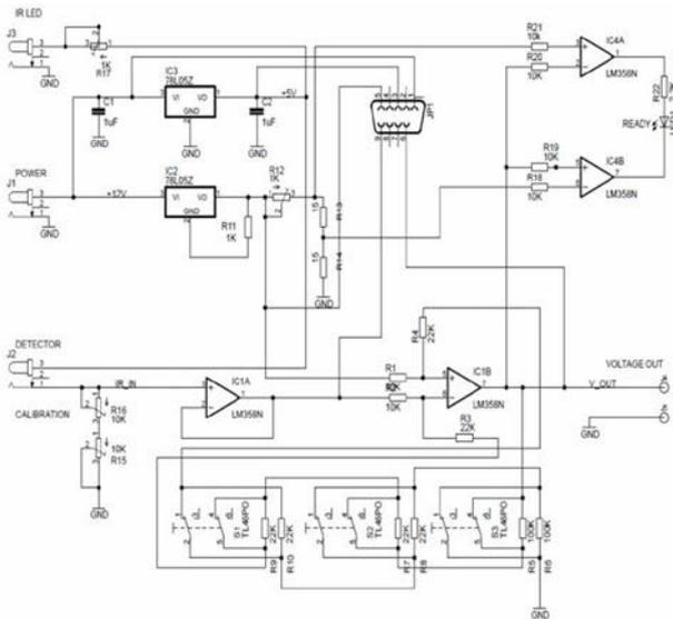
Fig. 2 – Electrical schematic of Fog Detector 1.
