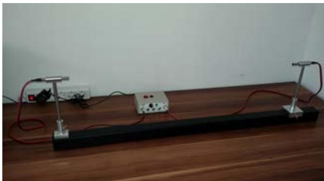
Fig. 6 – Measuring setup for Fog Detector 1.
