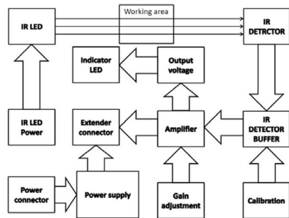
Fig. 1 Block diagram of Fog Detector 1.
