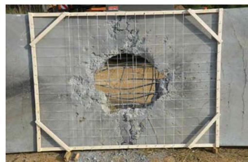
Fig. 2 Timber frame with string grid to experiment data evaluation.
